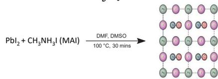
Figure 3. Synthesis scheme for MAPbI<sub>3</sub><sup>3</sup>.
