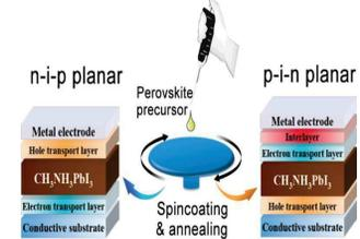
Figure 8. Visual of MAPbI<sub>3</sub> device stack structures<sup>4</sup>.
