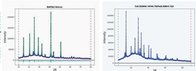
Figure 5. X-ray diffraction (XRD) patterns of perovskite films. Left: BSU. Right: NREL.
