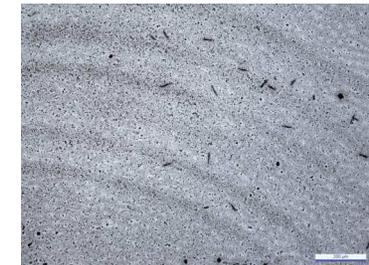
Figure 9. Optical microscopy image of triple cation thin film synthesized at BSU.
