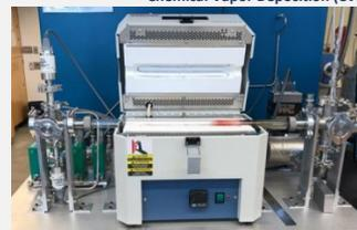
1. Nickel foam is placed in the furnace where it is heated in a vacuum and exposed to methane gas.
