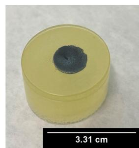
Figure 8: Sintered pellet mounted in epoxy for characterization
