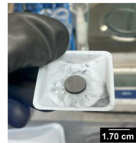
Figure 5: ZrC green pellet. The pellet is 12.70 mm in diameter.
