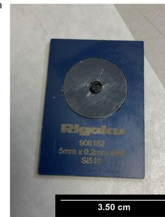
Figure 10: ZrC + vacuum grease on XRD stage
