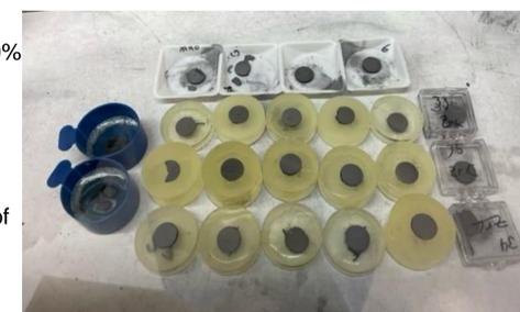
Figure 15: ZrC pellets mounted in epoxy have been sintered
