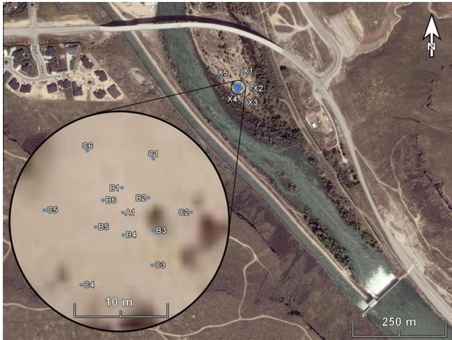
Fig. 1. Map showing location of the Boise Hydrogeophysical Research Site relative to Boise river. Site coordinates: 43°32'33.5"N, 116°5'50.5"W. Inset shows layout of wells in the central area of the site (figure from Cardiff et al. (2012)).
