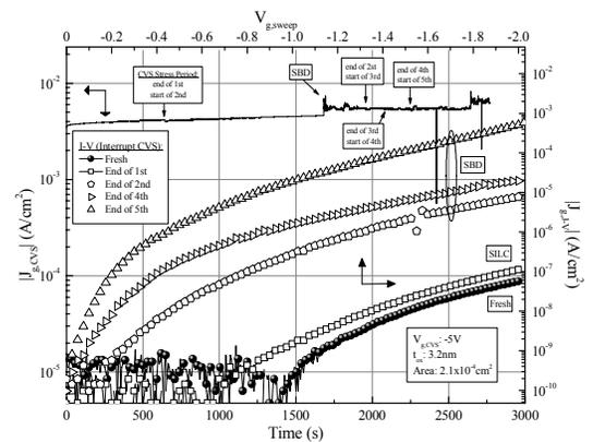
**Figure 4:** CVS J-t plot showing SBD and the intervals in which J-V measurements were performed. Corresponding J-V plots demonstrating SILC and SBD (symbol every 5 points).
