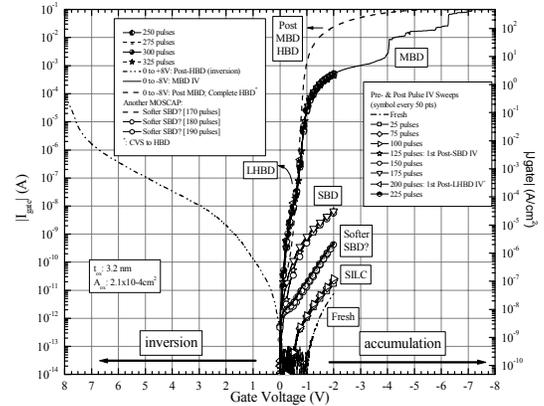
**Figure 2:** Similar to figure 1, but in addition, showing MBD and asymmetry of the I-V data with regards to inversion versus accumulation following HBD.
