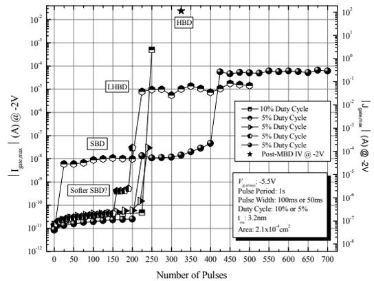
**Figure 3:** Current at -2V versus number of pulses at 5 and 10% duty cycles. Evident is SILC, soft SBD, SBD and LHBD. HBD after MBD is shown for comparison.
