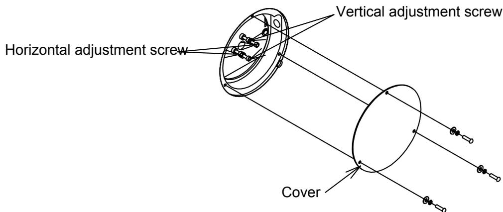
Fig. 4.4 Mirror adjustment screw
