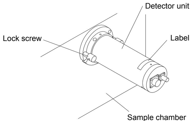
Fig. 2.6 Installation of detector unit
