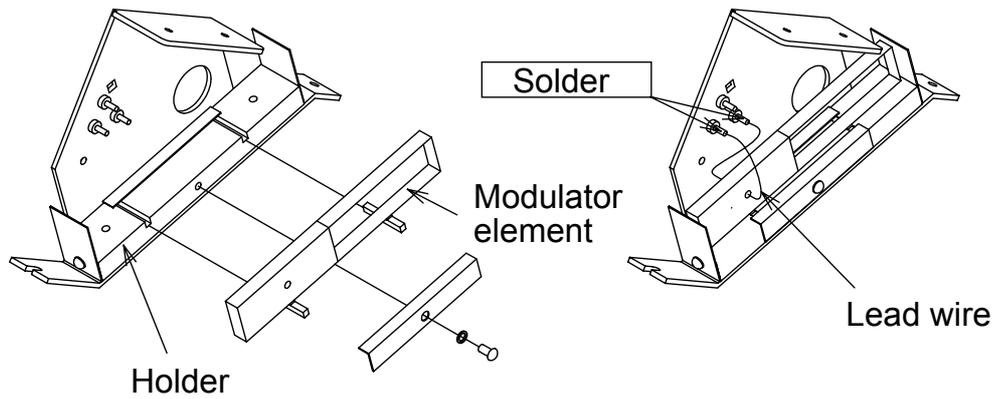
Fig. 2.5 Mounting the modulator element
