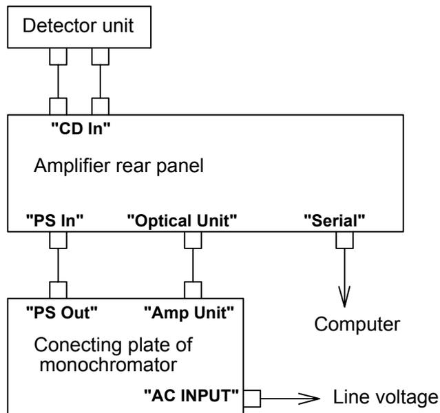
Fig. 2.7 Connection of cables
