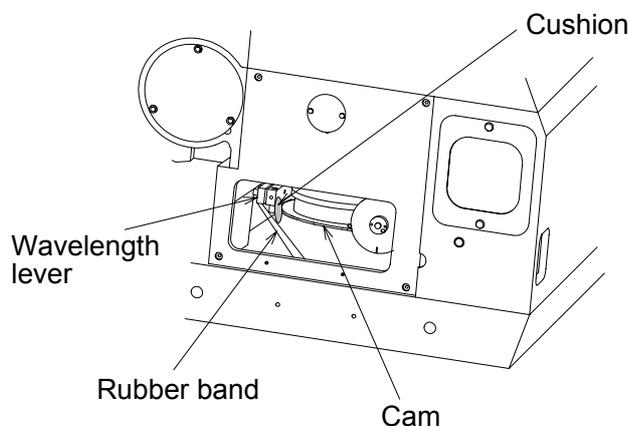
Fig. 2.2 Removing the cushion and rubber band
