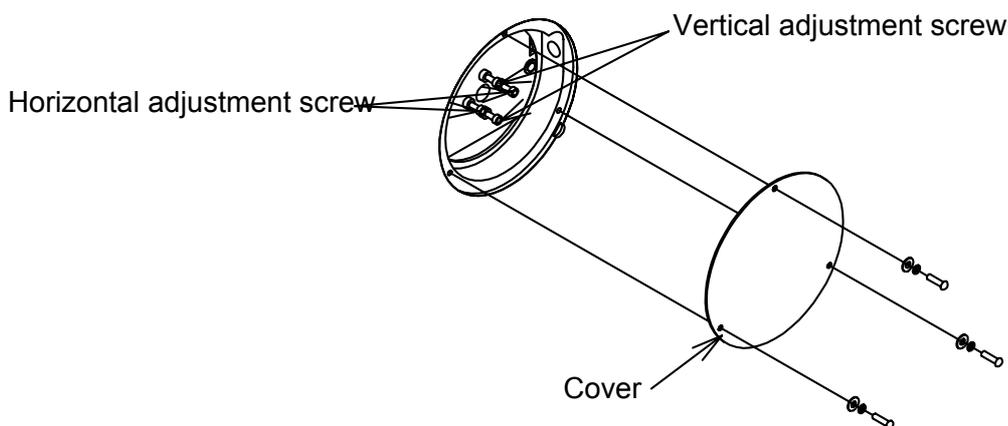
Fig. 4.4 Mirror adjustment screw
