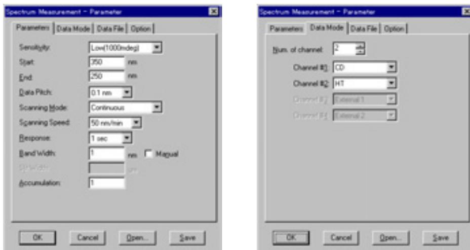
Fig. 4.11 Measurement parameters (CD scale check)
