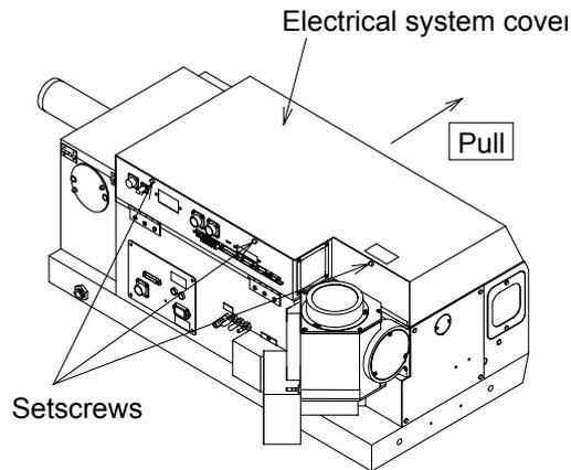
Fig. 2.3 Removing the electrical system cover
