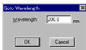
Fig. 4.7 Setting wavelength (energy check at 200 nm)
