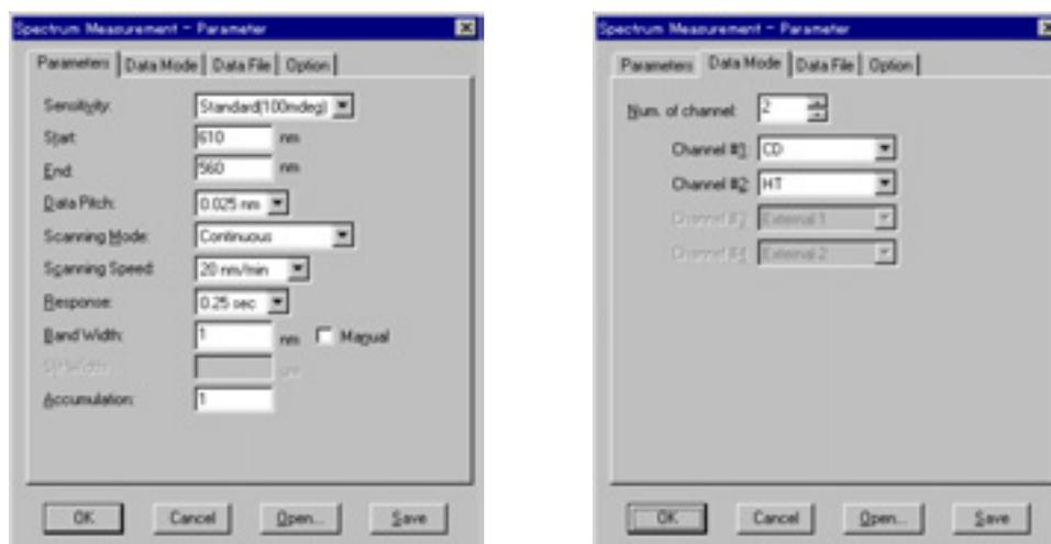
Fig. 4.8 Measurement parameters (wavelength accuracy check)
