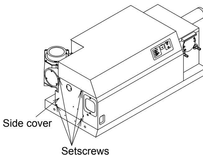
Fig. 2.1 Removing the side cover
