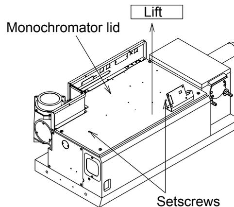
Fig. 2.4 Opening the monochromator lid
