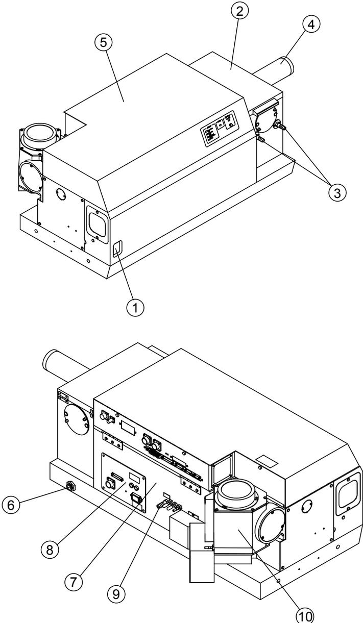
Fig. 3.1 Overall view (150 kW light source. Small sample chamber)
