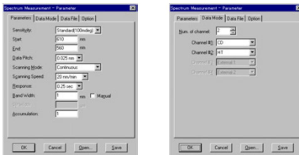
Fig. 4.8 Measurement parameters (wavelength accuracy check)
