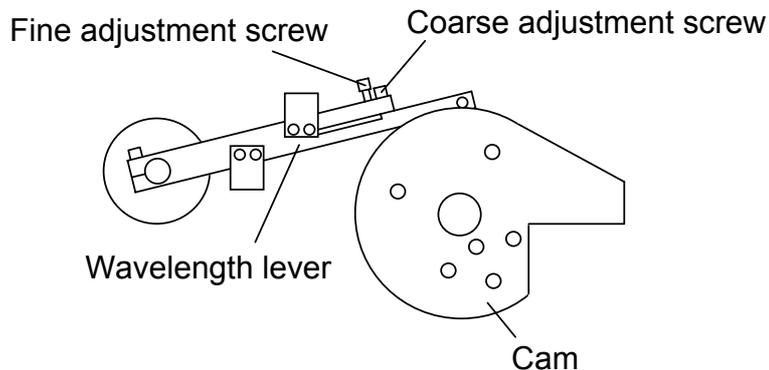
Fig. 4.10 Adjustment screws
