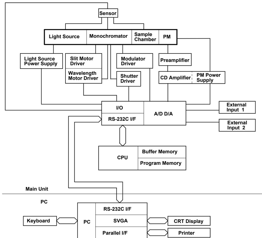
Fig. 1.3 Block diagram of electrical system
