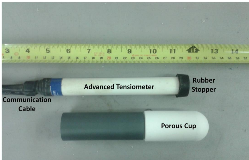
Figure 2: Advanced Tensiometer sensor and porous cup.
