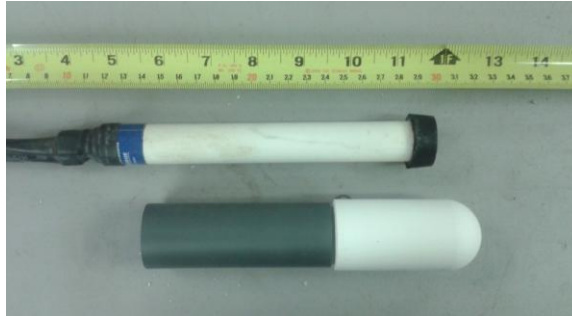
Figure 2-8: Advanced Tensiometer sensor (top) and porous ceramic cup (bottom).
