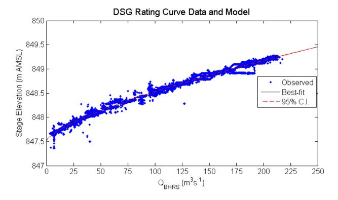
Figure 7: DSG rating curve data from 2009 – 2011 and best-fit line with 95% confidence interval (C. I.) on predicted measurements.
