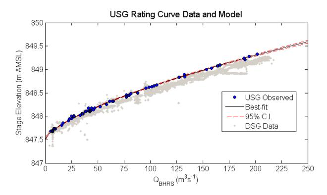
Figure 8: USG rating curve for 2009 – 2011 visual staff gauge data and best-fit line. Shaded points are the DSG data for comparison.
