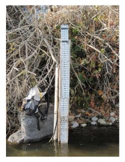
Figure 4: Downstream river staff gauge and stilling well at low stage, gauge increments are 0.02 ft.
