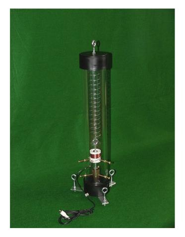
The original Slinky vertical seismometer was encased in 3" ABS plumbing pipe.
