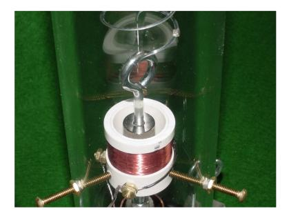
The damper plate could be a cylinder ring of aluminum, 1"id x 1.5"od x .750" tall.
