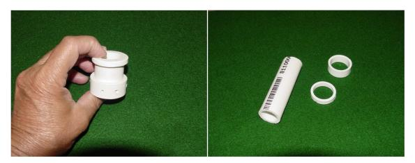
The coil body is 1" id and 1.75" in overall length. It is made of PVC plumbing fittings, cut to fit. Note: Use any 1" pvc fitting, like a coupler for the rings. Use the thinner wall pvc pipe, 200 psi, and not the thicker pipe, for the body.
