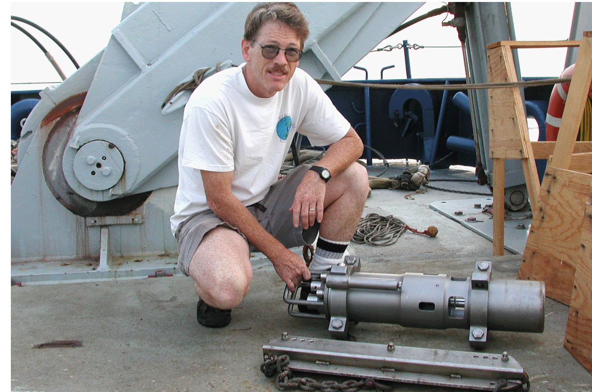
Figure 2: Seth Mogk and one of the 150 c.i. GI guns used for seismic sources on NEMO-3.
