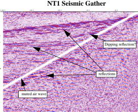
FIGURE 4. (A) The trailer-mounted seismic source used for the seismic reflection project. (B) Annotated shot gather from site NT1 along the downtown railroad spur near Orchard Road. Processing includes f-k and 40-150 Hz spectral whitening filters and air wave mute and shows the data quality of the raw field records.
