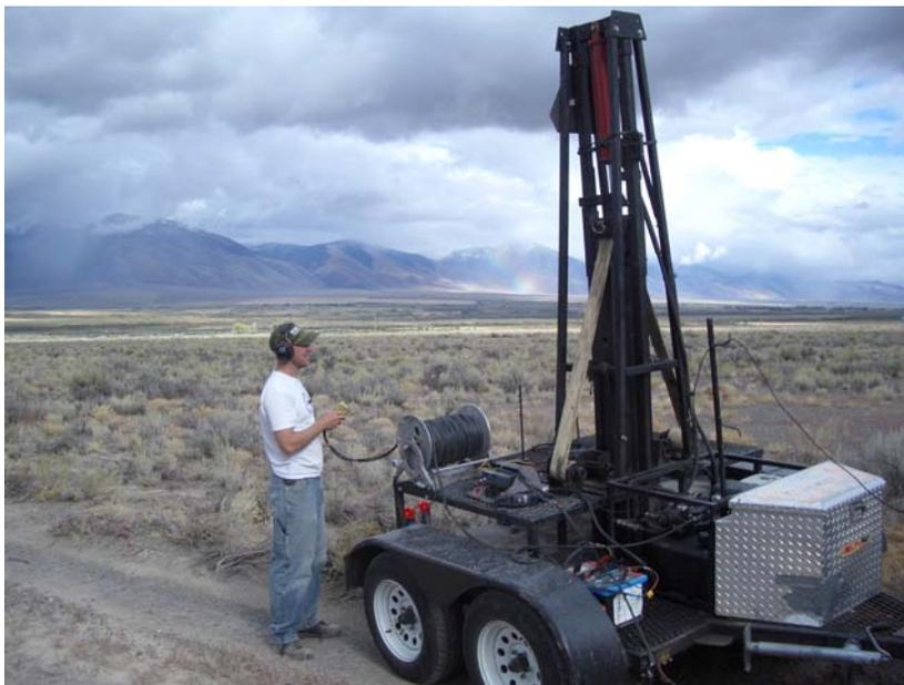
**Figure 3. Seismic source along Morgan Creek alluvial fan.**
