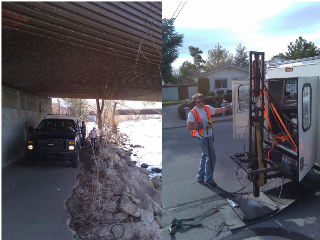
Figure 2. (left) Boise State seismic source truck beneath the East 2 nd Street bridge along the Truckee River seismic profile. (right) University of Nevada Reno student Brady Flinchum operating the controls of the hitch-mounted Boise State seismic source along the Warren Way seismic profile.
