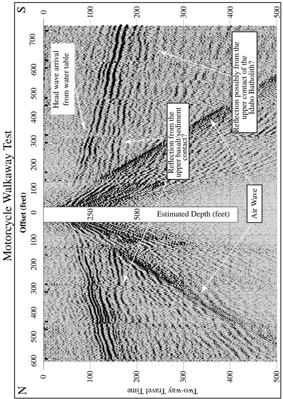
**Figure 3**. EWG walkaway results from the Motorcycle walkaway test. Note the reflection interpreted from the upper basalt contact and the weaker reflection deeper in the section possibly from the upper contact of the Idaho Batholith. Additional reflections in the upper section may also be present, but difficult to image due to the recording environment.
