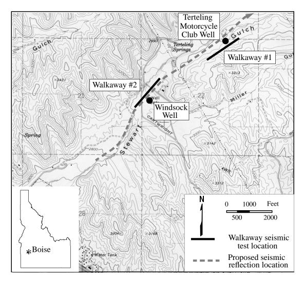
**Figure 1**. Topographic map of the field site northwest of downtown Boise. Walkaway locations and proposed seismic line location are shown.
