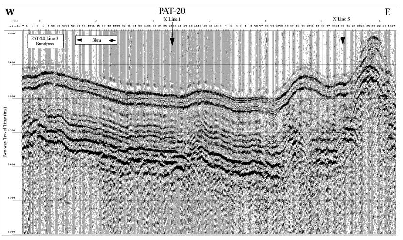
Figure PAT20-3: Western part of the seismic profile PAT20-seisline 3, across the proposed drillsite, from EW9709.
