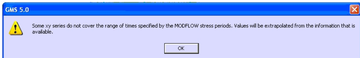
Figure 47: Error message 1: Error message associated with assigning stress periods to the model
