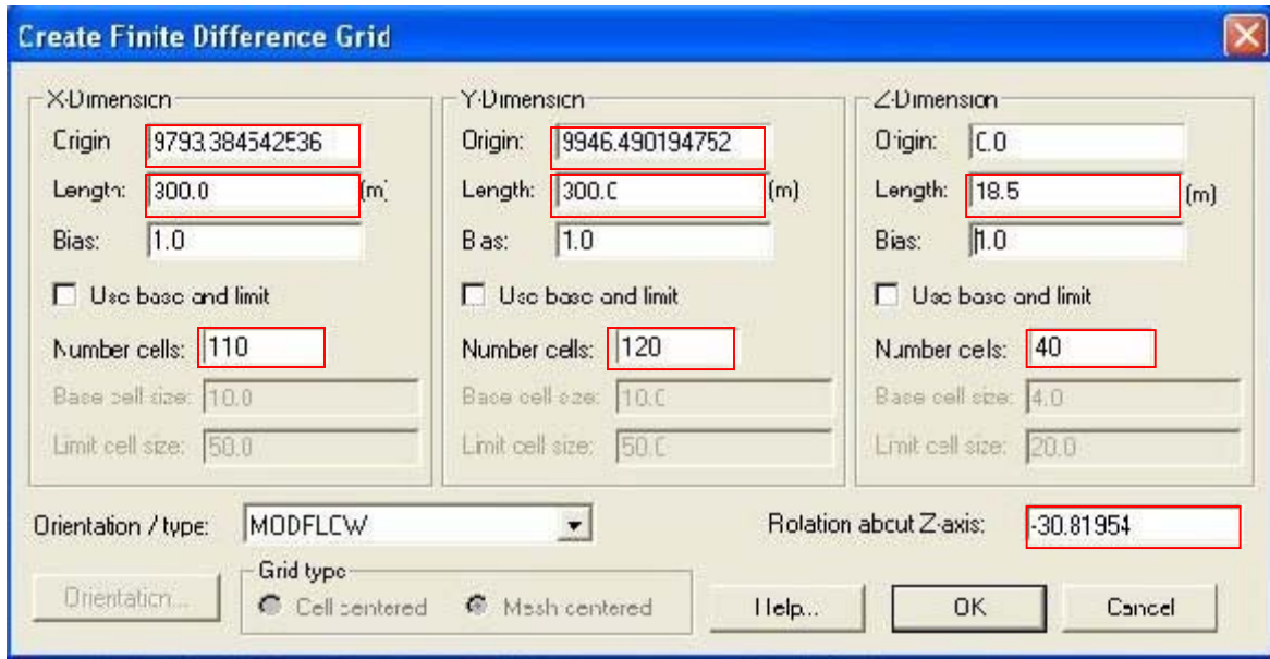
Figure 54: Create Finite Difference Grid dialog box showing appropriate values for the flow and transport model
