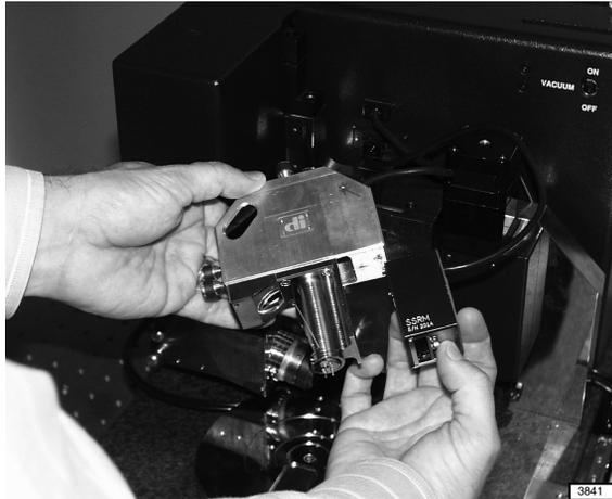
**Figure 289.5b:** Installed Application Module
