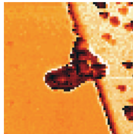
Figure 5. Adhesion map of the platinum/glass interface of Figure 3. Lighter pixels represent greater adhesion. The map was constructed by plotting the minimum value of each retracting curve at its x-y position. Note the variation of adhesion across the interface.
