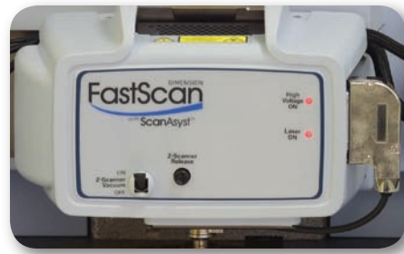
Scanner Resonant Frequency X-Y: 2.70kHz, Z: >50kHz.
