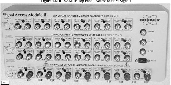
Figure 12.1b SAMIII: Top Panel, Access to SPM Signals
