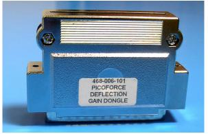
Figure 13.5g PicoForce Deflection Gain Dongle (PDGD) (468-006-101)
