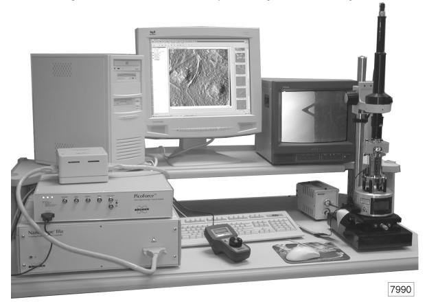
Figure 3.2c The MulitMode PicoForce System with Optional OMV Video Optics
