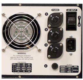
Figure 9.1b Fuse Holders on the Back of the NanoScope V Controller
