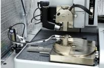
b. **Dimension Icon**: Place the water and gas lines on the stand-off holding the heater/cooler to the Dimension Icon chuck base. See Figure 4.2p.
