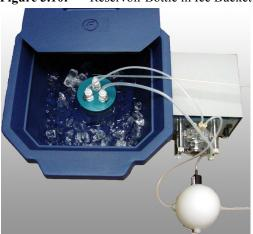
Figure 3.10r Reservoir Bottle in Ice Bucket
