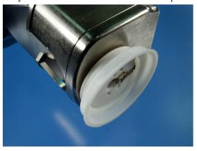
6. Align the laser beam to reflect into the photodetector from the tip-end of the cantilever (refer to the appropriate *Dimension Scanning Probe Microscope Instruction Manual* for detail).
