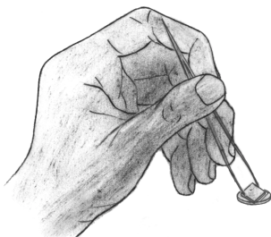
Figure 7.3k Securing Double-sided Tape to the Sample Disk
