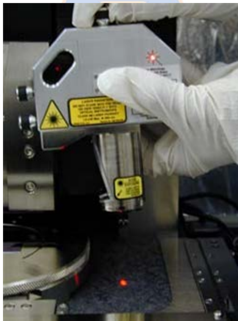
Figure 7. Alignment of the laser onto the AFM probe cantilever.
