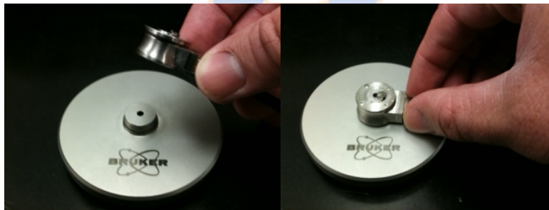
Figure 9. FastScan Z-scanner (probe holder) and mounting block.
