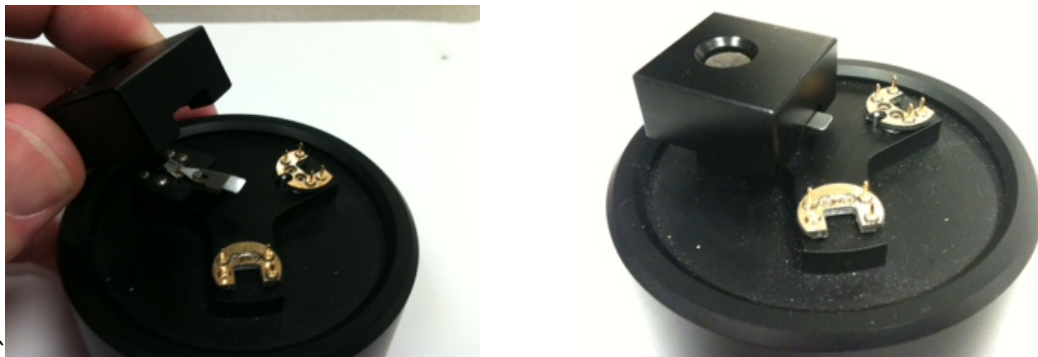
Figure 4. Magnetizing an MFM probe.
