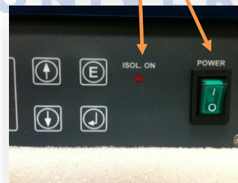
Figure 1. Power strip for Multimode (left) and controls for Herzan active vibration isolation table (right).
