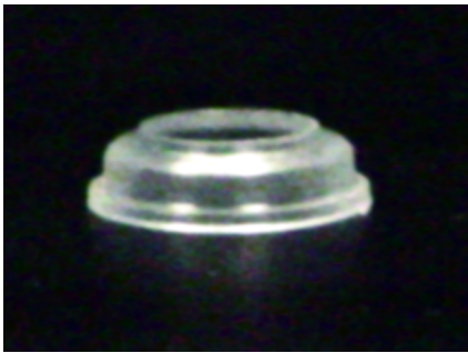
Silicone O-ring showing "S"-shaped profile.
