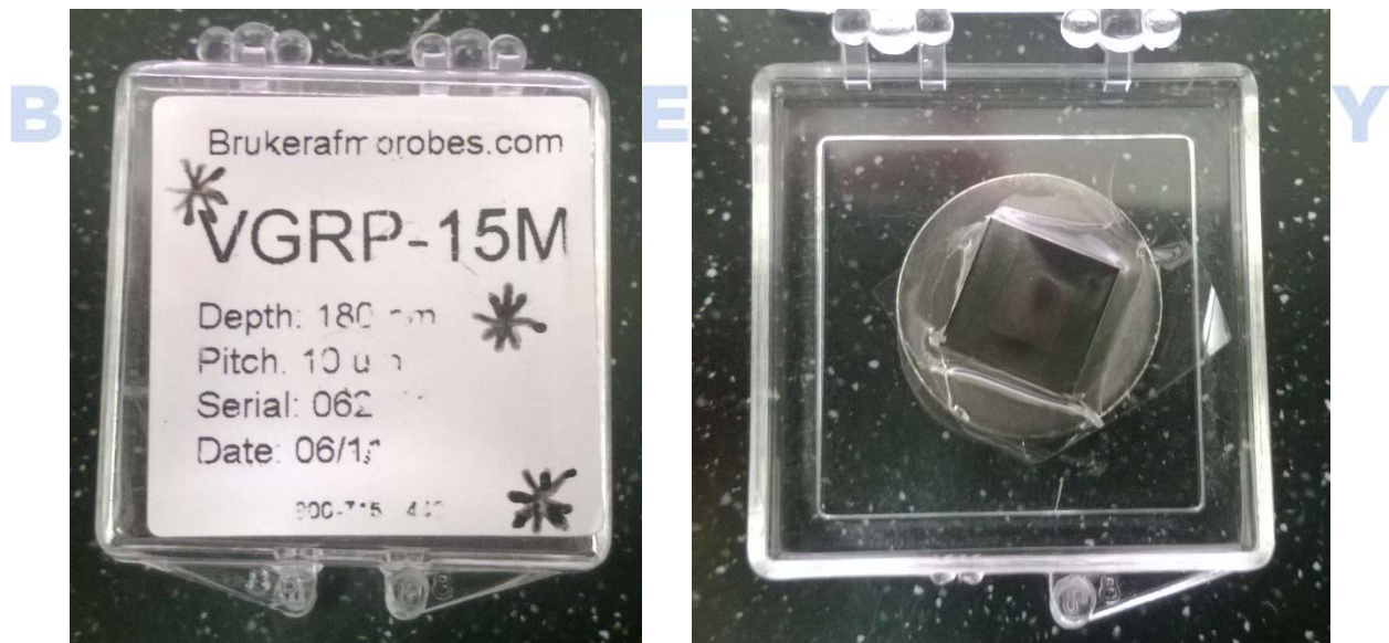
Figure 3. The VGRP-15M calibration reference box marked with black asterisks (left), and VGRP-15M calibration reference covered with a thin film of cellulose replicating tape (right).
