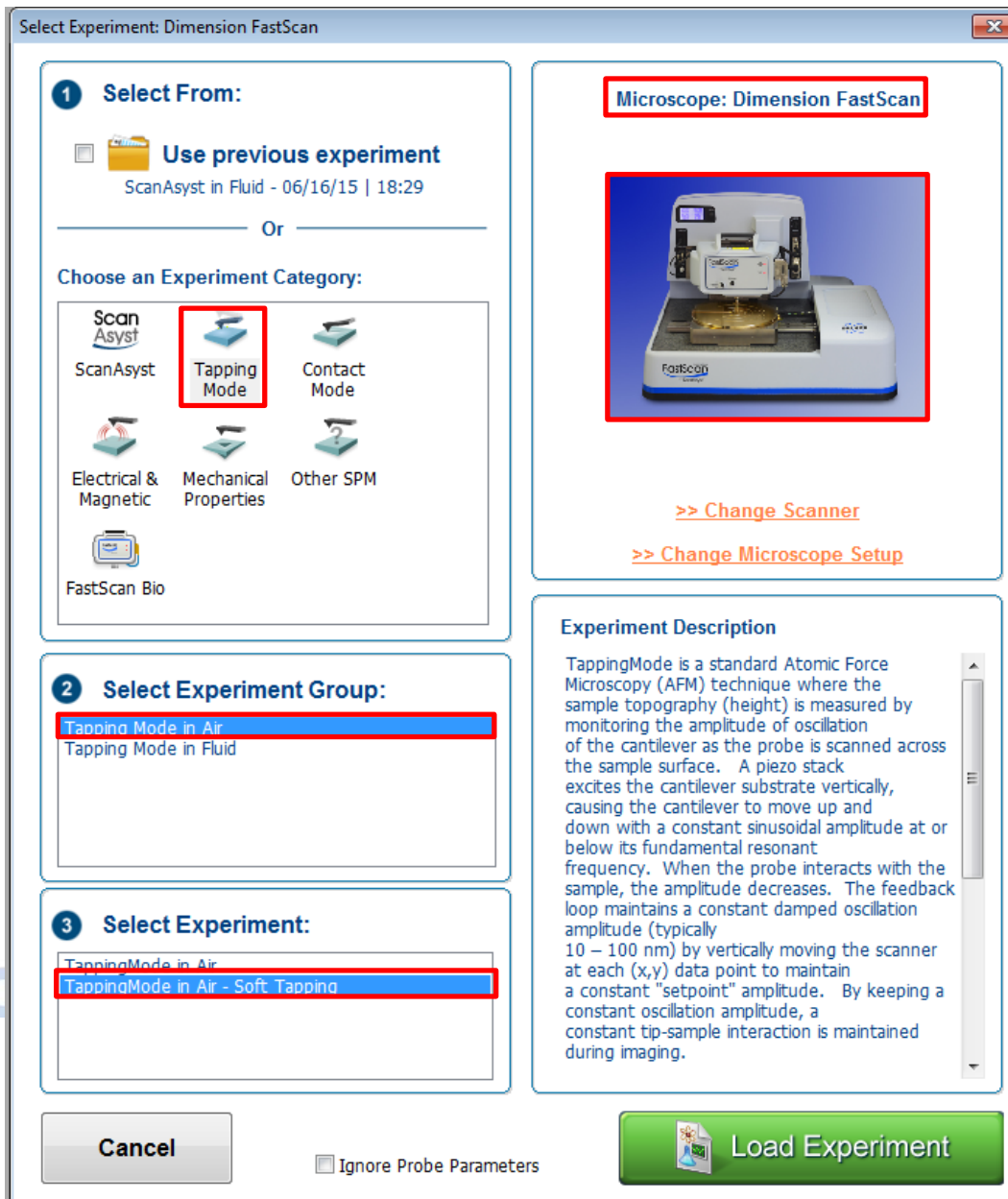
Figure 1. The Select Experiment interface with the Microscope Select window opened indicating the Dimension FastScan head is selected. Red boxes highlight the proper experiment type and AFM selections.
