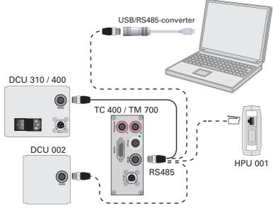
Fig. 3: Optional connection possibilities for interface RS485
