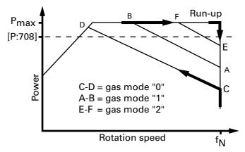
Fig. 4: Principle of power characteristics lines for gas type dependent operations, e.g. gas mode = 0
