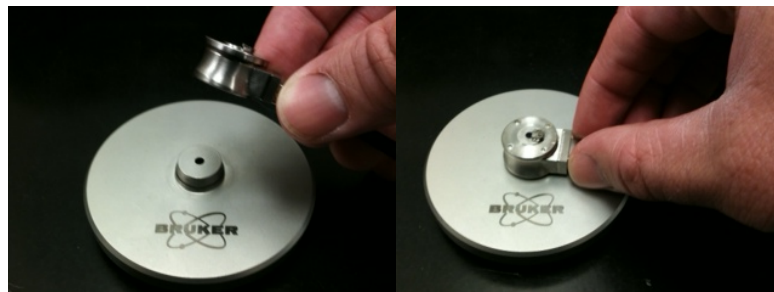
Figure 1. The FastScan probe holder (also known as the FastScan Z scanner) and probe holder mounting block for the Dimension FastScan AFM.
