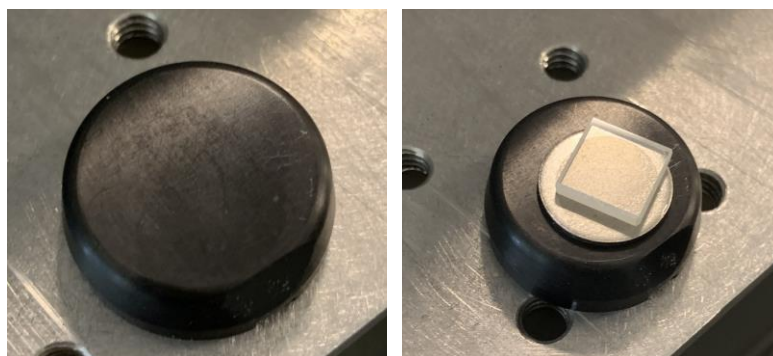
Figure 5-8: A sample holder (left) and a sample mounted on a sample holder (right)
