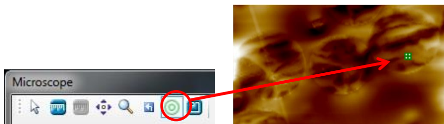
Figure 4-8: The Target icon on the Microscope window (left) and the AFM probe location on the AFM image (right) here on a PMMA bead in the test sample
