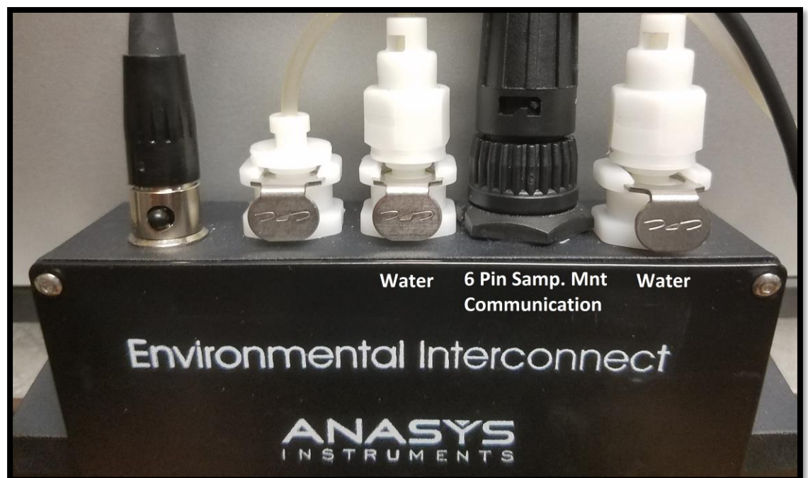
Figure 10-4: The remaining connections for the environmental interconnect. The Water hoses are bipolar, and it is recommended to route them such that they are not mechanically restricted.
