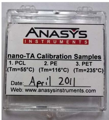
Figure 4-1: Calibration Sample kit.
