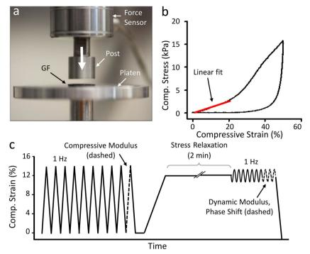
**Figure 3.** Mechanical characterization protocol of GF and GF-tissue composites. a) The testing apparatus was assembled to compress the GF with homemade compression platens. b) A typical stress–strain curve for GF displays elastic behavior between 0% and 14% compressive strain. c) The testing method designed to measure the quasi-static and viscoelastic compressive properties of GF with and without cell culture (not drawn to scale).
