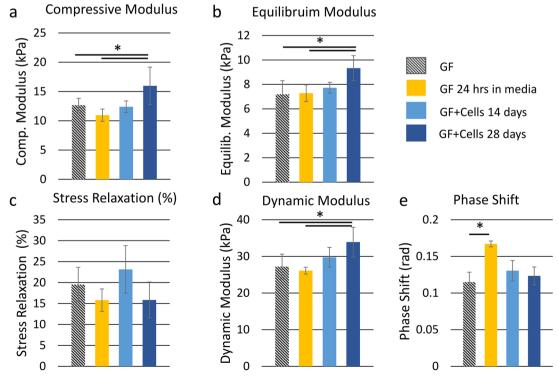
Figure 4. The measured quasi-static a), b) and viscoelastic c–e) properties of conditioned graphene foam (GF), graphene foam after 14 days of cell culture in chondrogenic medium (GF+C 14 days) and graphene foam after 28 days of cell culture in chondrogenic medium (GF+C 28 days).
