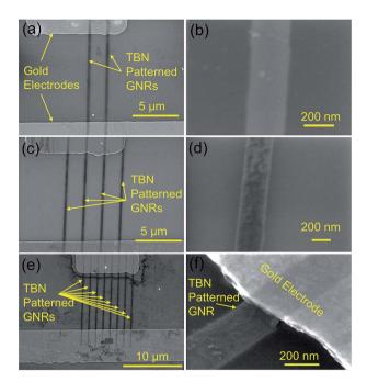
**Fig. 5** SEM images of different arrays of TBN-fabricated GNRs across Au electrodes. (a) an array of 2 parallel GNRs across Au electrodes; (b) zoomed-in view of one GNR; (c) an array of 4 parallel GNRs across Au electrodes; (d) zoomed-in view of one GNR; (e) an array of 8 parallel GNRs across Au electrodes; (f) a zoomed-in view of intersection of GNR with a Au electrode.
