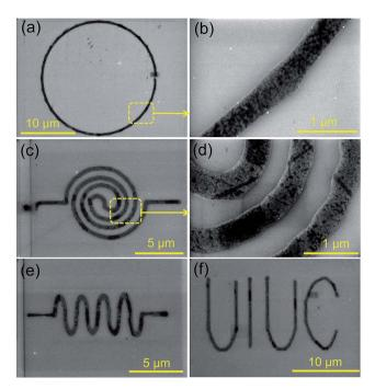
Fig. 4 SEM Images of different shapes of TBN-fabricated GNRs, demonstrating the fabrication flexibility of this TBN method. (a) A circular GNR with a radius of 10  $\mu$ m; (b) a zoomed-in view of a section of the circular GNR; (c) a spiral-shaped GNR; (d) a zoomed-in view of a section of the spiral-shaped GNR; (e) a wavy-shaped GNR; (f) GNR forming the shape of "UIUC" representing University of Illinois at Urbana-Champaign.
