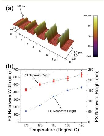
**Fig. 2** (a) 3D AFM height image of PS NWs deposited using different temperatures but with the same tip speed of 150 nm s<sup>1</sup>; (b) measured widths and heights of PS NWs deposited using different temperatures but with the same tip speed of 150 nm s<sup>1</sup>.
