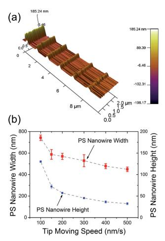
Fig. 3 (a) 3D AFM height image of PS NWs deposited using different tip speed but with the same temperature of 175 C; (b) measured width and height of PS NWs deposited using different tip speeds but at the same tip temperature of 175 C.
