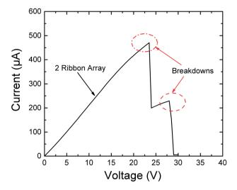
Fig. 8 Breakdown characteristics of 2 ribbon array. 2 breakdown levels are observed indicating the sequential breakdown of multiple ribbons. The calculated maximum current density is of the order of  $10^8$  A cm<sup>2</sup> which is consistent with literature-reported values.
