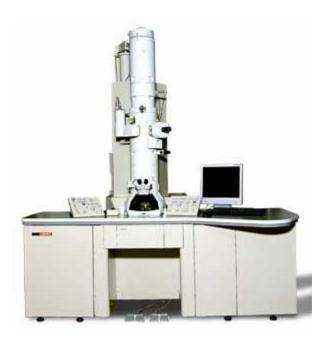
EDS and EELS Chemical analysis Post column annular dark field detector Tomography unit for 3D images In situ heating and cooling: 77 K to 1000 C ASTAR orientation mapping and precession electron diffraction
