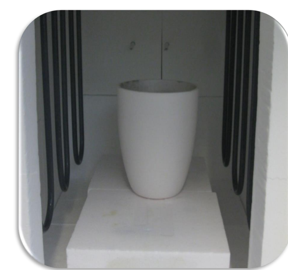
Figure 6: Crucible in furnace during calcining process
