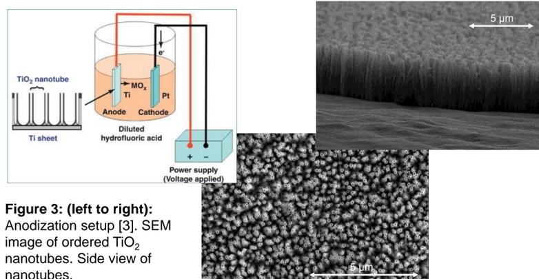
Figure 3: (left to right): Anodization setup [3]. SEM image of ordered TiO<sub>2</sub> nanotubes. Side view of nanotubes.
