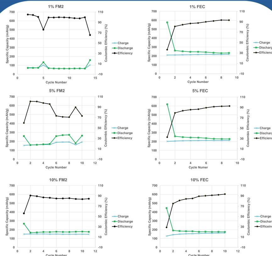
Figure 6: Electrochemical data from cycled cells.
