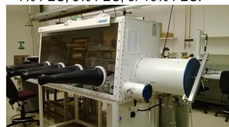
Figure 4: Argon glove box where electrolytes and coin cells were prepared.
