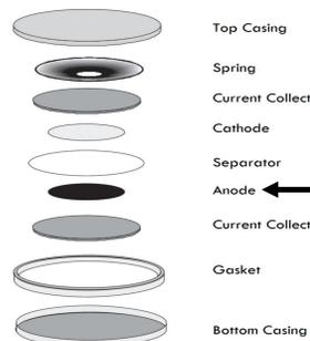
Figure 5: Construction of coin cells.
