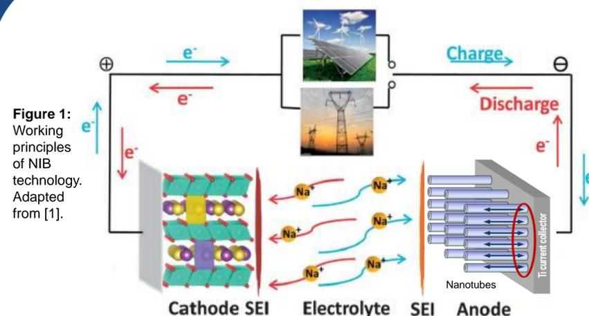
Figure 1: Working principles of NIB technology. Adapted from [1].
