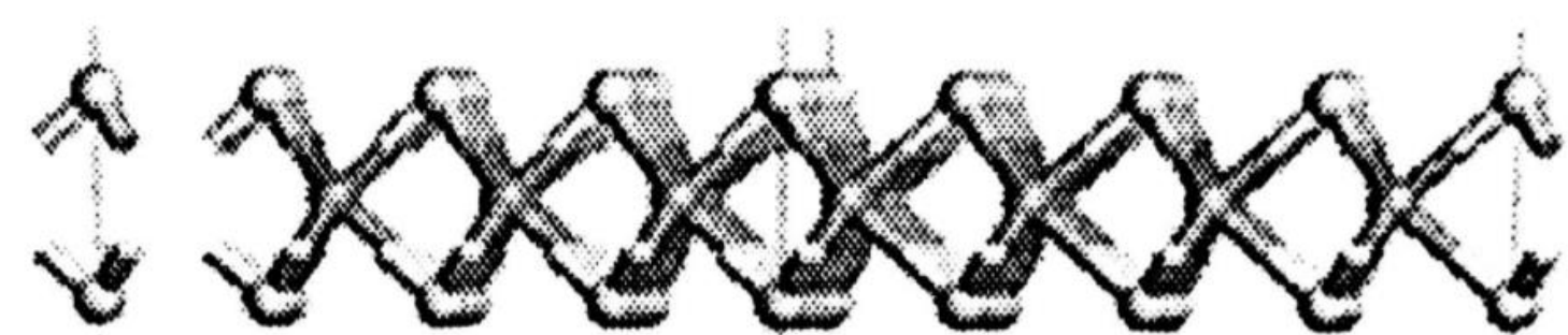
Fig 1. Layered X-M-X atomic structure of MX 2 along c-axis. M is shown in blue, and S in yellow. Adjacent layers (not shown) form with weak van der Waals interactions.
