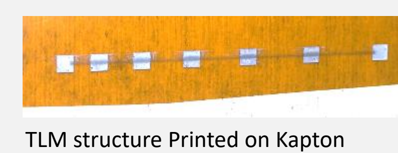
TLM structure Printed on Kapton
