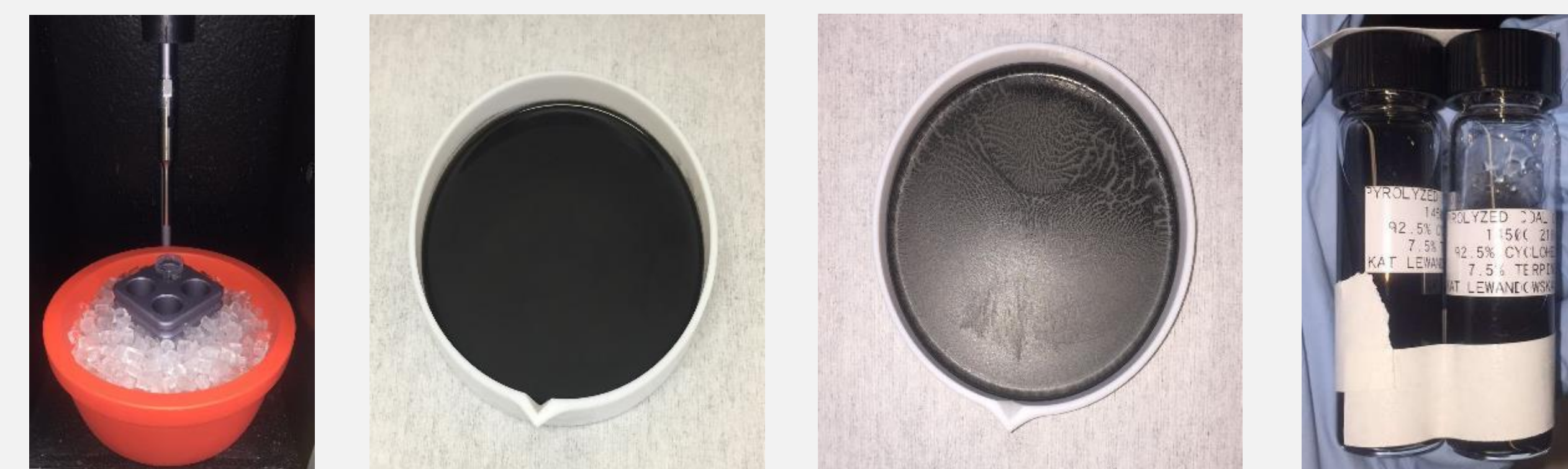
Ink solution chilled in an ice bath while sonication
