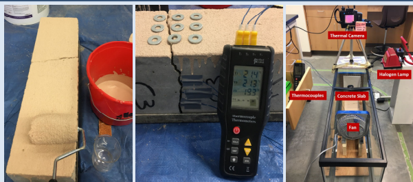
Figure 5. Various steps in the experimental setup, including coating application, point selection and data collection for the wind environment.
