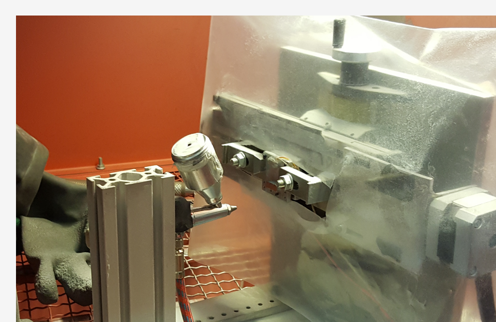
Figure 5: A image of the micro-peening equipment used for the experiment.
