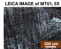
Figure 3. LEICA optical microscopy image of MT01. Directional solidification and dendrites are evident.
